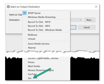
Configure the Zixi destination with the Broadcaster IP address, Ports, & Channel Name (Stream ID) from the Broadcaster configuration above.
