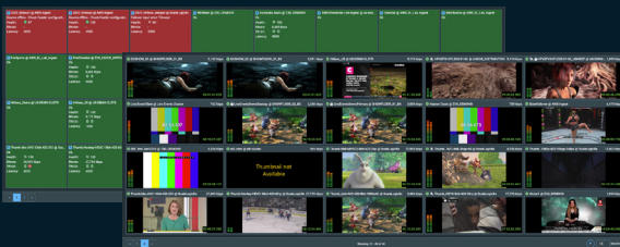
Customizable ZEN Master GRID Views dynamically sort channels based on health, providing 'at-a-glance' actionable insights.
