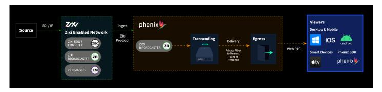
Customer streams can be ingested into Zixi Broadcaster. Once processed, the streams are handed over to the Phenix Encoder which feeds the Phenix Cloud via Phenix's Interactive Transport Protocol (ITP). A WebRTC stream is then generated and distributed to clients using Phenix's standard output methods utilizing resilient infrastructure and multi-cloud architecture.
